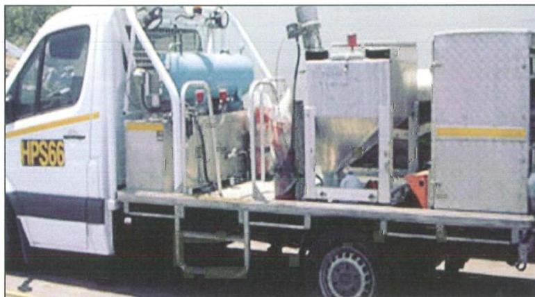
Figure 12 – Improved fixed step with hand rails.
