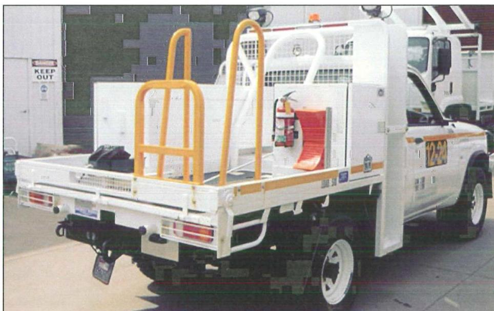
Figure 13 – Drop down tray side with integrated step.
